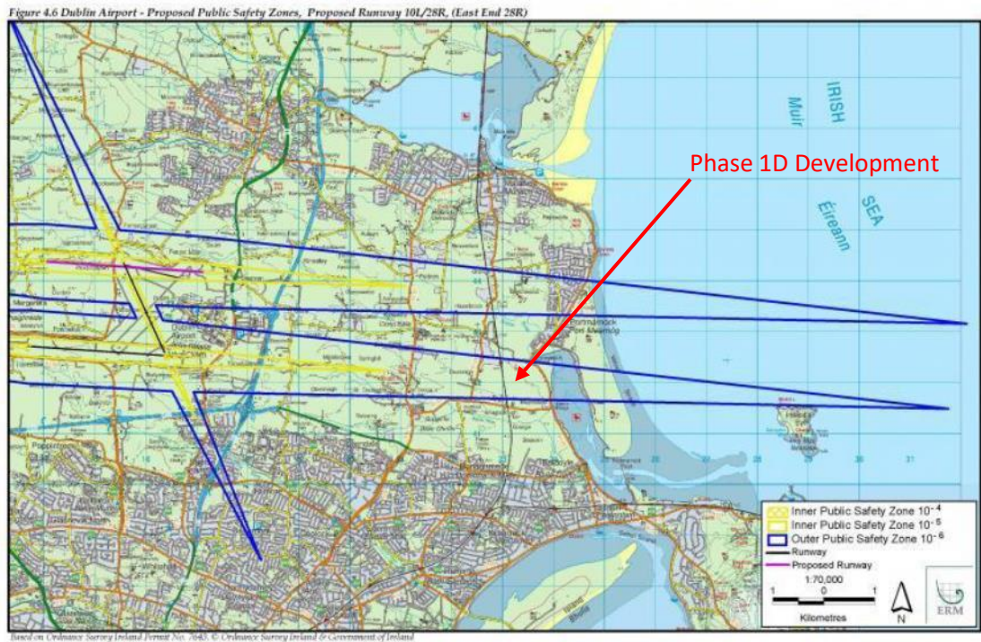
Figure 3:PSZ at Dublin Airport
